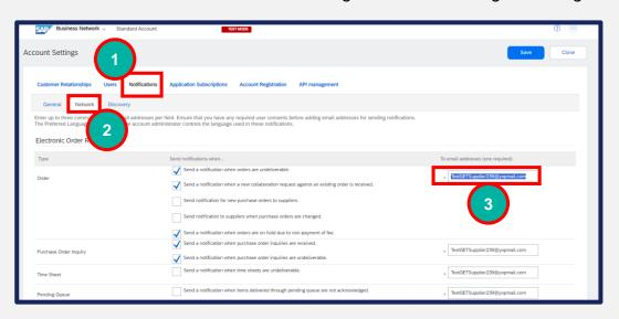
You can enter up to **five** email addresses per the notification type. Separate each address with a comma but NO space between the emails.
